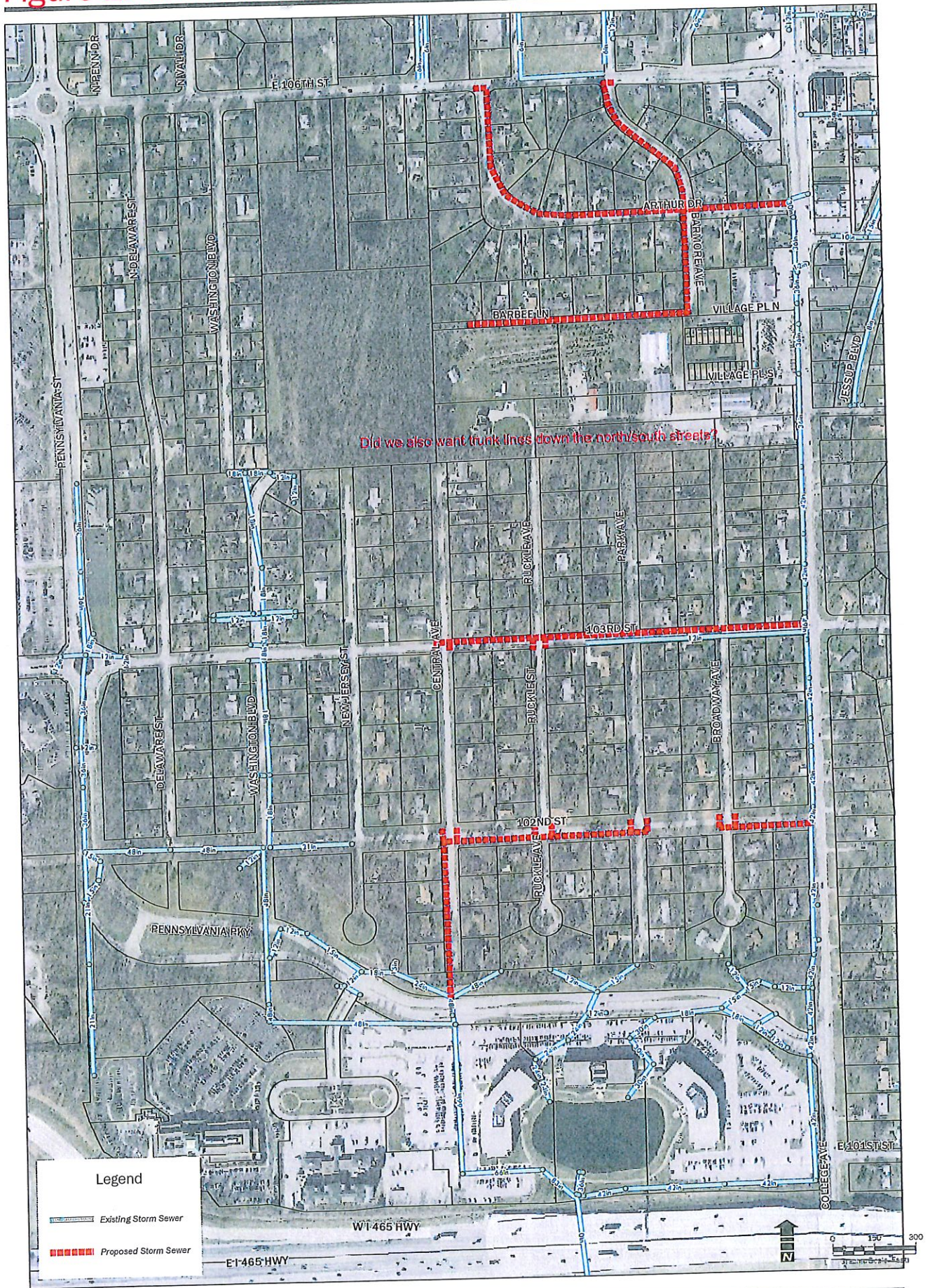
Figure 1: Clara Knotts Drain Stormwater Improvements
